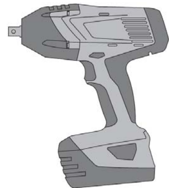
Install the screw anchor by impact screw driver Hilti SIW 22T-A or SIW22-A
