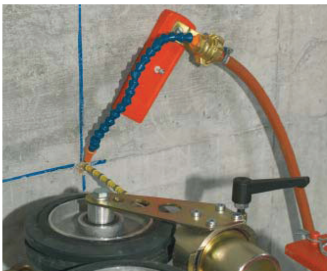
Mount the cooling water nozzles.
