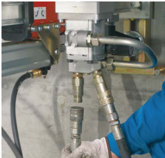
Connect the hydraulic hoses to the drive unit.
