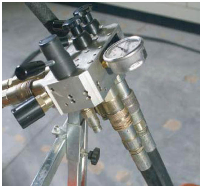
Connect the hydraulic hoses to the drive unit.
