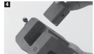
4 Insert the breech into the marking head and secure the locking screws M6x30 with an Allen key.
