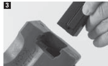
3 After placing the absorber on the impact extractor insert them into the marking head as shown.
