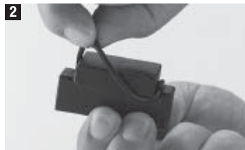
2 Mount a new rubber O ring on the impact extractor as shown.
