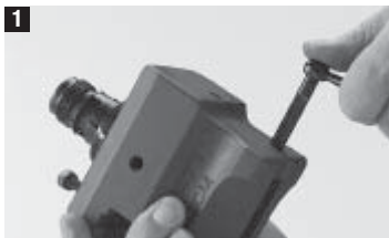
1 Insert the axle with locking lever in the bore as shown and firmly press it until it clicks into place.
